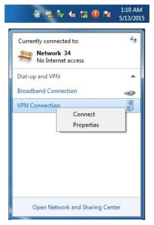
② Click Properties > Security, set the Type of VPN to Point to Point Tunneling
